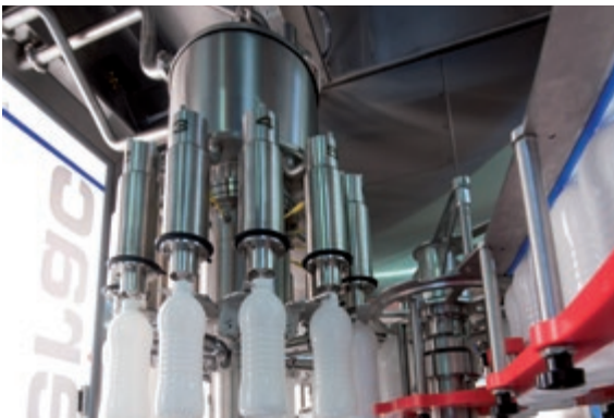
H2F filling turret with a sloped casing
