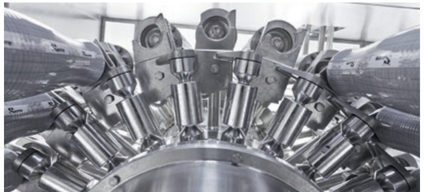
EHEDG designed load cell in the H2F filling turret
