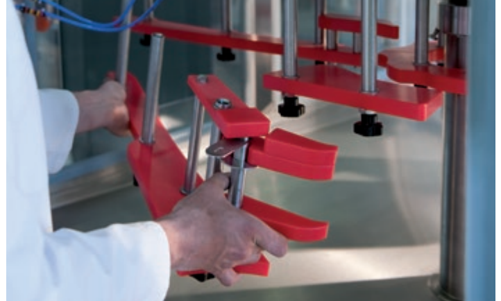
Very fast tool changes in the filling zone
