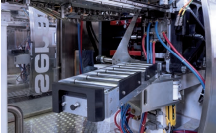
Mold sliding rack for easy and effortless changeover
