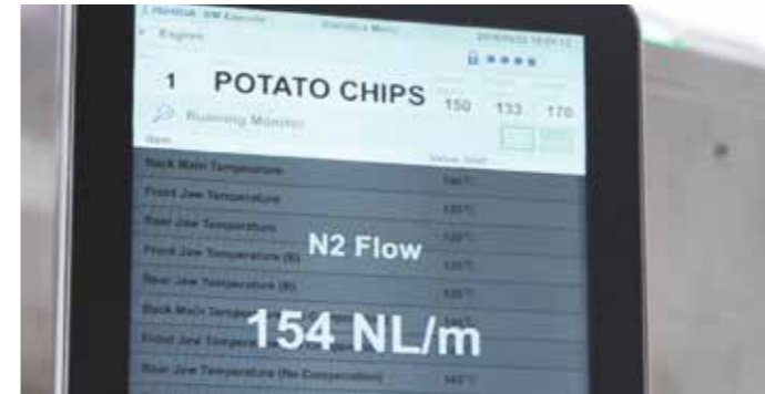
An inbuilt flow meter combined with an electro-pneumatic controlled valve, allows for the precise delivery of nitrogen to each pack, as defined by the preset configuration, minimising nitrogen waste whilst maintaining pack seal performance.
