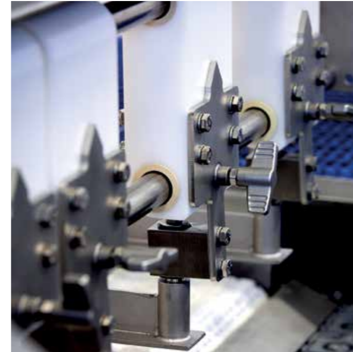
No tools needed for dismantling
