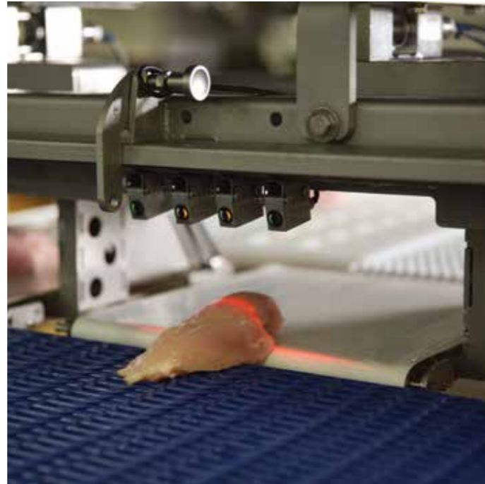
Simple, reliable orientation determination based on photocells
