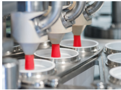
Volumetric filling (up to three filling stations possible)
