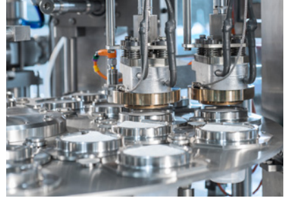
Pre-formed cups heat sealing
