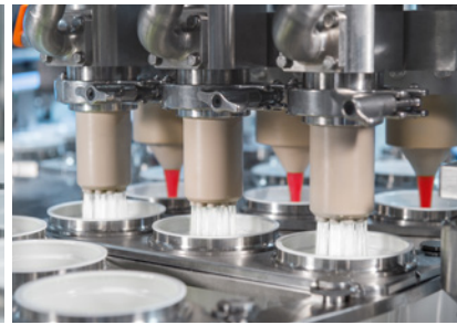
NEO machine equipped with two filling stations
